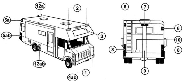
Figure 7 - Bus Illustration for § 393.11 8 (5ab) (12ab) 9 (4ab)
