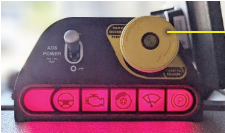
Figure 4. Emergency Manual Override (EMO)
