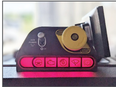
Figure 11. Emergency Manual Override (EMO)
