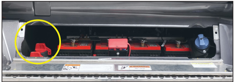
Driver step hatch with battery bank and disconnects
