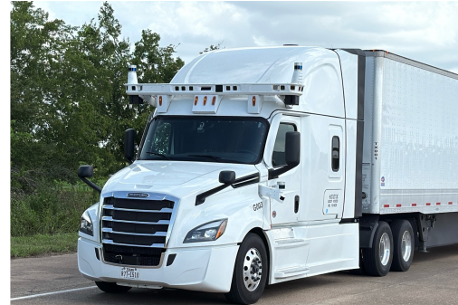
Figure 1: Bot Auto Truck with sensor array
