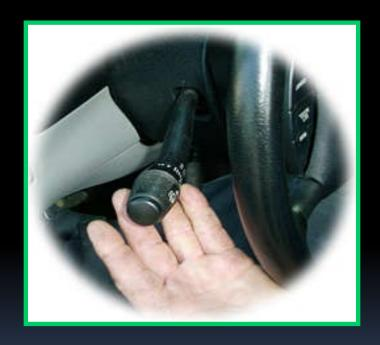
Remember: Selector switch must lock in proper turn position when applied but need not cancel automatically.
