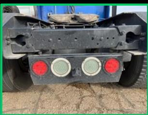
Turn signal lamps: required on all vehicles beginning 1960 or newer (2 in front, white or amber; 2 in rear, red or amber); turn signal lamps on the front of the truck-tractor that are two-faced and visible to the rear will not be rejected or failed for not having no rear turn signals.
