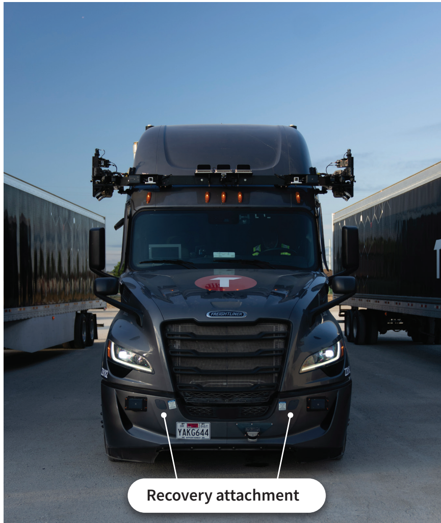
Figure 21. Recovery hook attachment locations
