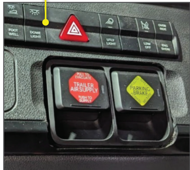
Figure 6. Parking brake switches
