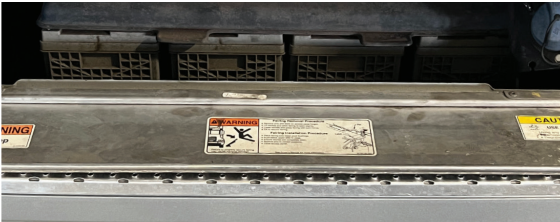
Figure 19. Driver-side panel, showing location of batteries
