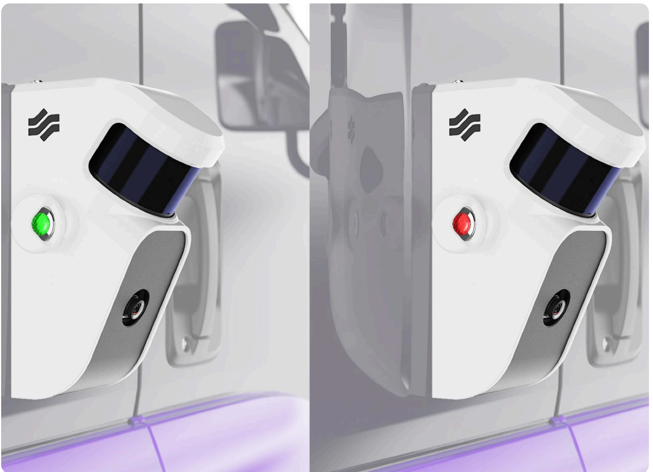
Figure: ADS Indicator Light States - ADS immobilized, safe to approach (Green) and ADS engaged, not safe to approach (Red)
