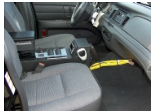
Above and to the left: Special wiring harnesses allowed fleet workers to quickly install communications equipment in new patrol vehicles.
