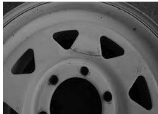
Cracked Wheel/Hand Holds
